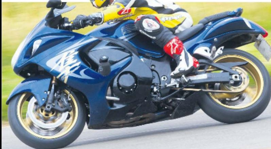
MCN's Trevor Franklin on the TTS Hayabusa. The foam next to the crash bung is the supercharger air intake
