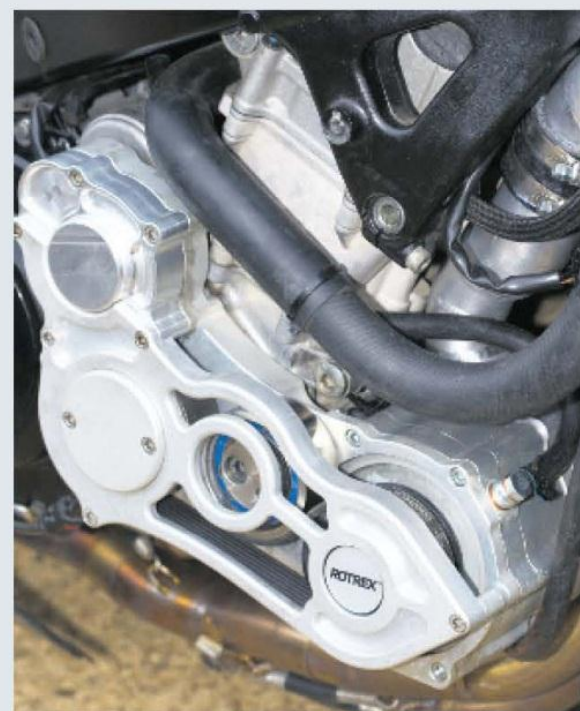
Drivebelt takes power from the crank to spin the supercharger
